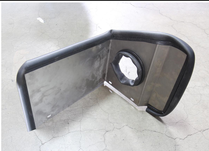
12. Install the provided bubble edge trims onto the heat-shield in the areas shown above.
