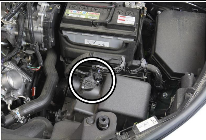
6. Disconnect the Mass Air Flow sensor connector from the MAF sensor.
