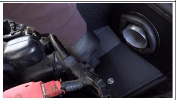
22. Remove the air duct hose from the resonator.
