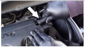
20. Insert and secure the provided EPDM hose along with the two EMSC-16-27 clamps onto the valve cover barb and intake barb.
