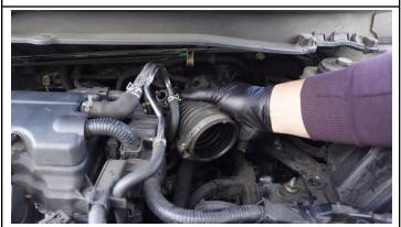
8. Remove the factory intake hose from the vehicle.
