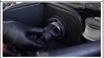
23. Insert the MAF sleeve into the intake pipe.
