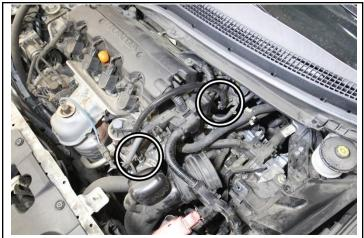
12. Install and secure the provided HTHH-032 heater hose along with the two FIC-12 clamps onto the coolant hose barbs.
