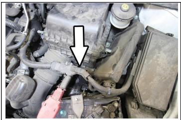
3. Unbolt the 10mm bolt securing the harness bracket and remove it from the vehicle.
