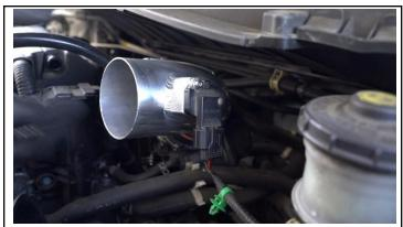
18. Connect the MAF sensor harness connector back onto the sensor.
