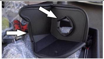
15. Attach the provided bubble edge trim onto the HPS heat shield.
