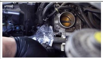
10. Using a plastic bag or container, carefully disconnect the coolant hose from the throttle into the bag to catch any coolant residue.
