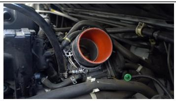
13. Insert the reducer coupler along with the provided T-bolt clamps onto the throttle body.
