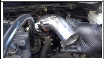
17. Insert the HPS intake pipe into the coupler, but do not secure the intake pipe at this time.
