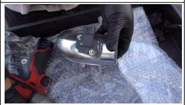
16. Insert and secure the MAF sensor onto the HPS intake pipe using the provided two M4 allen bolts.
