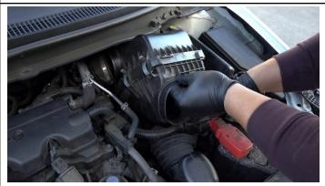
7. Carefully disconnect the air box assembly from the grommet and remove it from the vehicle.
