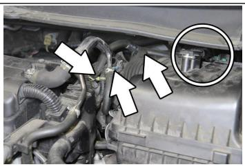
5. Loosen the hose clamp securing the intake hose from the throttle body. Disconnect the breather pipe from the intake hose and remove any vacuum hoses from the intake hose. Disconnect the MAF sensor harness connector and clip from the air box.
