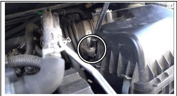
6. Loosen the hose clamp securing the intake hose from the upper air box assembly.
