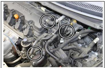
9. Loosen the hose clamps securing the throttle body coolant hoses and the breather hose on the valve cover.
