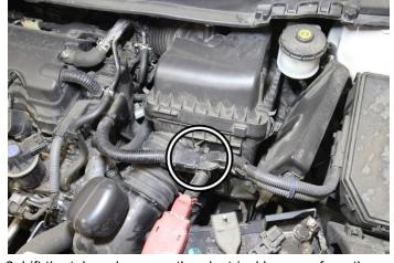
2. Lift the tab and remove the electrical harness from the bracket.
