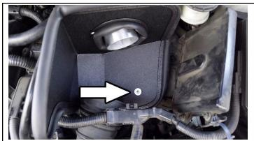
21. Once, the intake pipe and the heat shield are in the proper position secure the t-bolt clamp on the intake pipe. Secure the heat shield using provided M6 nut and washer onto the vibration mount.
