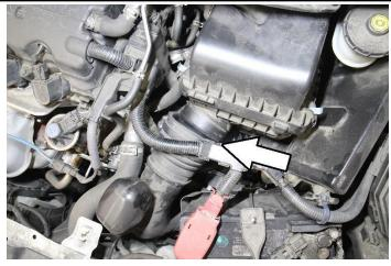
4. Disconnect the air duct hose from the lower air box assembly.
