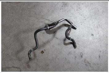
11. Remove the coolant hose and breather hose hardline assembly from the vehicle.
