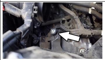
14. Insert the provided  $\frac{1}{2}$  vibration mount into the factory air box mount.
