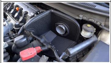
19. Insert the HPS heat shield into the vehicle.
