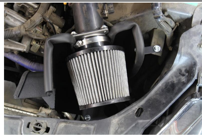
20. Insert the HPS performance air filter and reconnect the MAF sensor harness connector.
