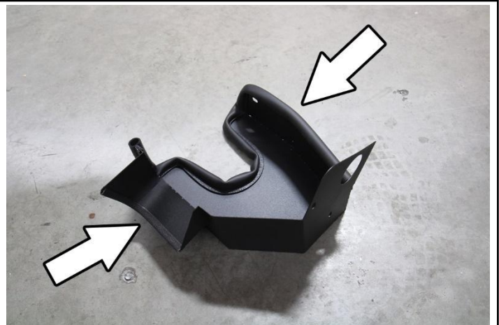
11. Insert the thin edge trim provided in the hardware kit indicated from the left arrow shown above onto the heat shield. Insert the bubble edge trim onto the heat shield indicated from the arrow on the right shown above.
