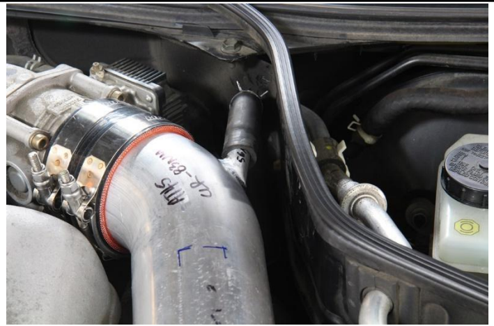
19. Insert and secure the factory breather hose onto the intake barb.
