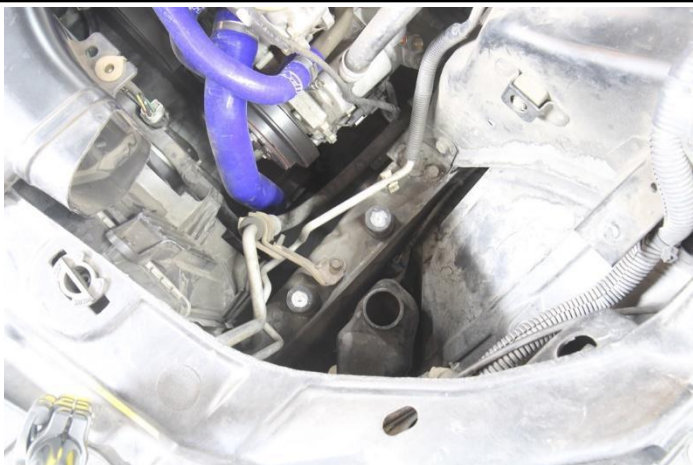
10. Insert the vibration mounts along with the M6 mounting bungs into the factory air box rubber grommet mounts.
