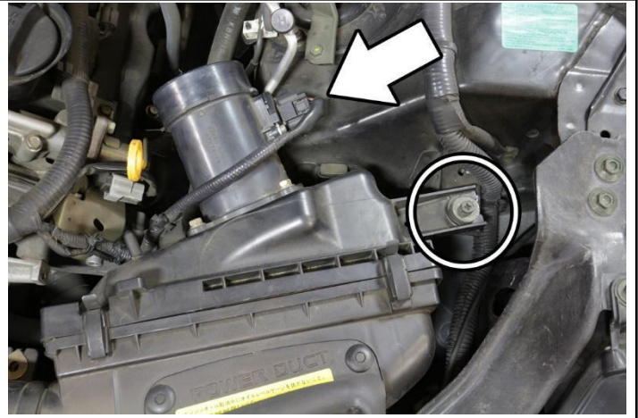
7. Disconnect the MAF sensor harness connector and remove the 10mm bolt securing the air box. Lift and remove the air box assembly from the grommets and remove the air box from the vehicle.
