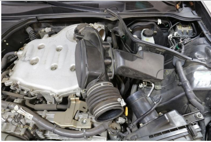
6. Remove the factory intake tube from the vehicle.
