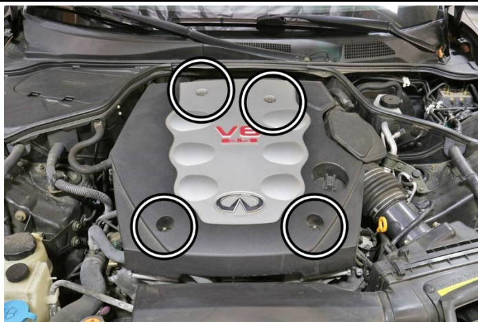
2. Remove the four 10mm nuts securing the engine cover and remove the engine cover from the vehicle.
