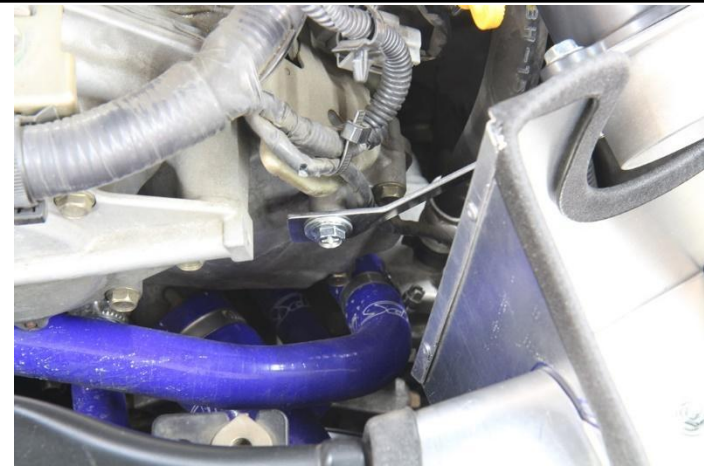
18. Once the intake pipe is adjusted into position, secure the intake bracket onto the mounting bolt that was removed in step 13.
