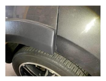
**STEP 18:** Re-apply fender flare to vehicle in best fit position.
