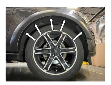
**STEP 7:** Apply pressure to the fender flare against the vehicle to create tension and begin to tighten all (5) mounting positions noted above.
