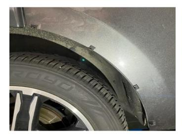
**STEP 25:** Slide push-on clip (X4) over the abrasion resistant tape in alignment of the slot in the fender flare
