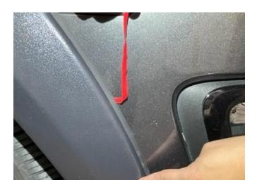
**STEP 8:** Once the fender flare is securely fastened to the vehicle, begin to pull the RED tape liner of the extrusion, and apply pressure to get the proper adhesion needed.
