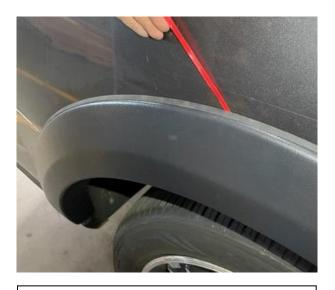
STEP 27: Once the fender flare is securely fastened to the vehicle, begin to pull the RED tape liner of the extrusion, and apply pressure to get the proper adhesion needed.
