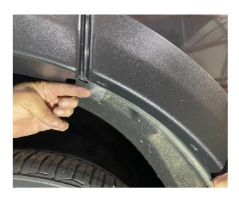
**STEP 24:** Place fender flare up against vehicle for best fit by aligning the end of fender flare with the doors edge as shown above. Align abrasion resistant tape with the (4) slots in fender flare. Remove fender flare.
