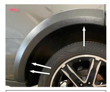
**STEP 23:** Apply pressure to the fender flare to create tension and begin to fasten.
