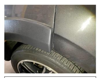
STEP 14: Place fender flare up against vehicle for best fit by aligning the end of fender flare with the doors edge. See above.
