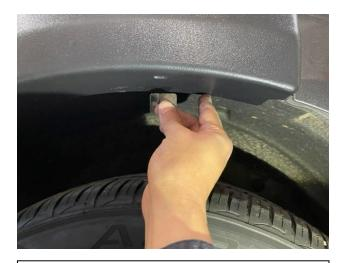
**STEP 15:** Align abrasion resistant tape with slot in fender flare. Remove fender flare.
