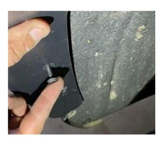
**STEP 20:** Begin to loosely install with long screws supplied in the hardware kit using 3mm Torx drive. Start at the upper position first.
