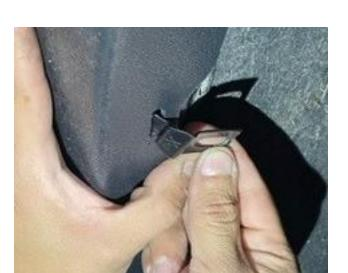
**STEP 5:** Secure attachment clips (X4) by sliding clip into Fender Flare slot. As shown above.
