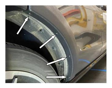
**STEP 26:** Apply pressure to the fender flare to create tension against the vehicle and begin to fasten all (4) mounting points as shown above. If slots are misaligned, you may need to adjust tape and clips accordingly when tightening.
