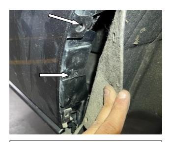
STEP 13: Note above the (2) positions U-Nut needs to be applied.
