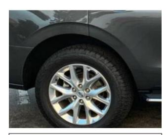
STEP 10: Using the alcohol wipes supplied, clean the body area where the Fender Flares will contact vehicle surface. Ensure fender surface is dry prior to install.
