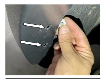
STEP 19: Place 5mm spacer behind the (2) slotted holes of the fender flare and begin to loosely install using the long screws supplied in the hardware kit.
