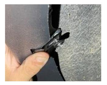
**STEP 5-1:** Using the factory screws that were previously removed, attach the clips to corresponding existing holes (X4) in upper inner wheel well. Do not fully tighten screws at this stage.
