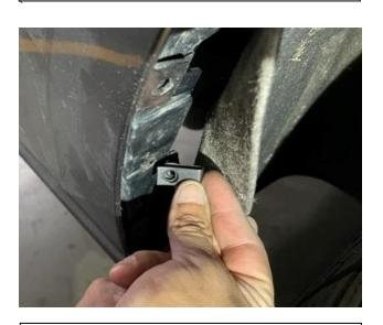
**STEP 12:** Install U-nut over existing hole of the hard plastic, not the tab of the painted surface.
