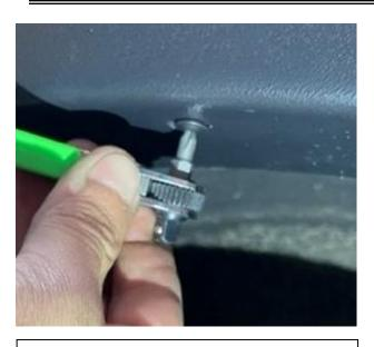
**STEP 22:** Use the small Philips screw that is provided in the hardware kit and loose fit the top center position.
