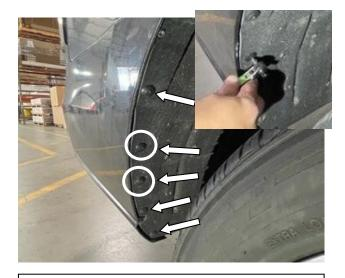
**STEP 11:** Remove the (5) push in fasteners for ease of installing the (2) U-Nuts. The U-nuts will be installed in the positions circled above.
