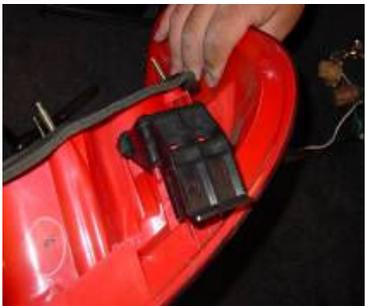
Step 16: Remove the clip located at the bottom of the stock taillight.
