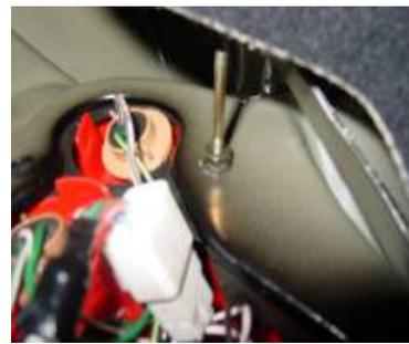
Step 12: Remove the 8 mm nut located at the top of the taillight assembly.
