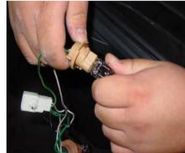
Step 15: Remove the two bulbs from the taillight sockets.
