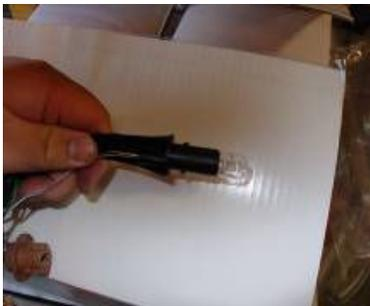
Note: Do not remove the bulb from the reverse light socket.
