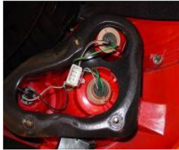
Step 14: Remove the wire harness from the taillight assembly.
