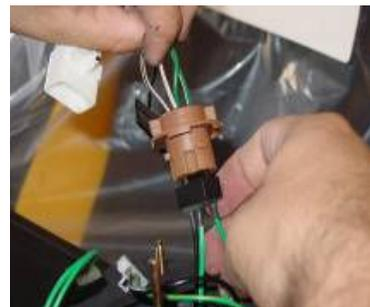
Step 20: Connect the pigtail from the taillight to the stock wire harness.
