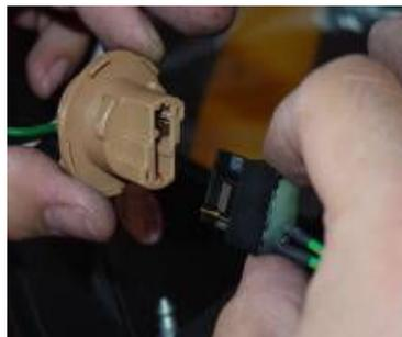
Step 19: Connect the pigtail from the taillight to the stock wire harness.
