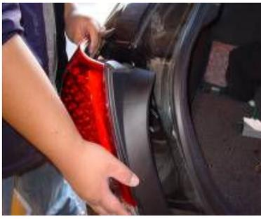
Step 21: slide the ANZO LED tail-light into place and check fitment.
