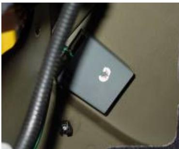
Step 18: Mount the resistor in a safe place where water will not get to it.
