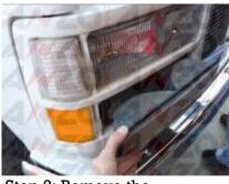
Step 2: Remove the parking lights from the vehicle.
