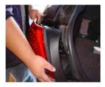
Step 21: slide the ANZO LED taillight into place and check fittment.
