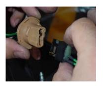
Step 19: Connect the pigtail from the taillight to the stock wire harness.
