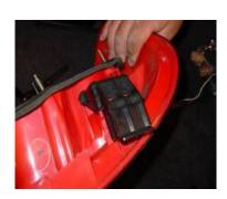
Step 16: Remove the clip located at the bottom of the stock taillight.
