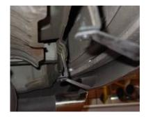
Step 5: Remove the plastic push pins located undernieth the bumper.
