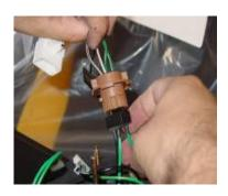
Step 20: Connect the pigtail from the taillight to the stock wire harness. Make sure to match the ground to
