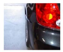
Step 7: Pull the side of the bumper off. Repeat step for passenger side.
