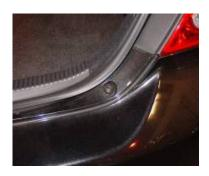
Step 1: Open the truck expossing the top of the bumper to remove the two phillip screws located at either end.
