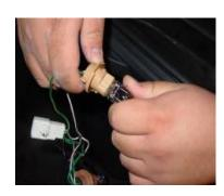
Step 15: Remove the two bulbs from the biege sockets.
